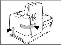
$\boldsymbol{2}$  While lowering the OPEN lever, open the reading unit.
